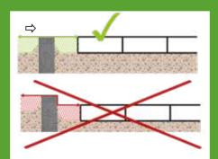
The ECORASTER<sup>®</sup> grid should be installed flush with the surface of the edge.
