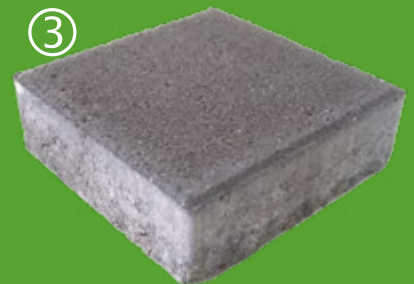
After weathering of limestone efflorescence
